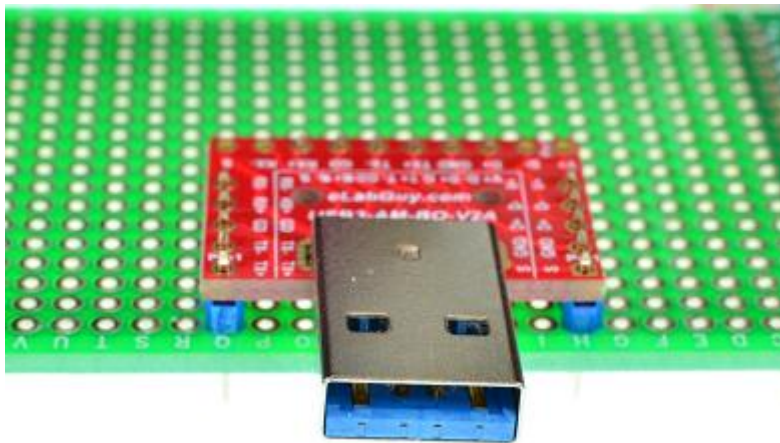
Figure 4: Solid Mounting on prototype PCB
